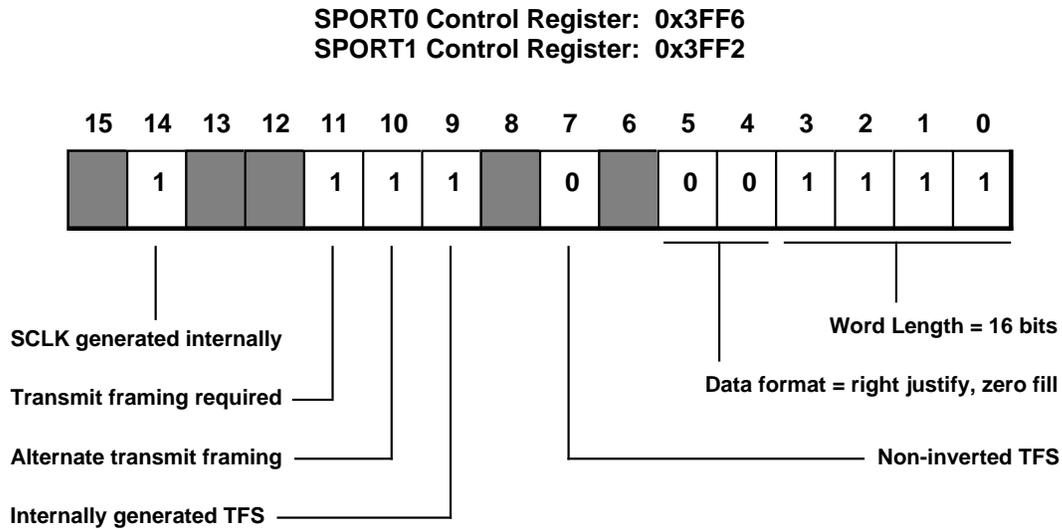
Figure 13.5 SPORT To AD766 DAC Control Register Settings
