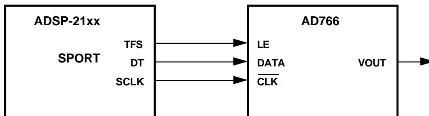
Figure 13.3 Serial Port Interface To AD766 DAC
