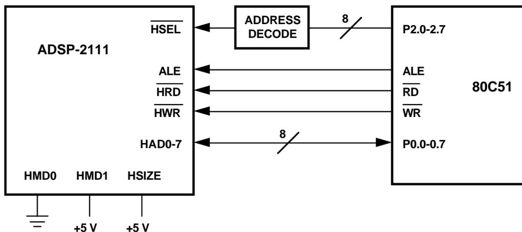
Figure 13.10 Host Port Interface to 80C51 Microcomputer
