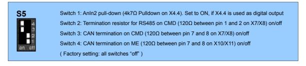
To activate the built-in termination resistors, switch 3 of S5 has to be set to ON.
