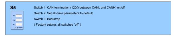
To activate the built-in termination resistors, switch 1 of S5 has to be set to ON.
