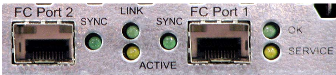
FIGURE 4-7. Built-In Hub, Showing the LEDs Located Between the Fibre Channels.
