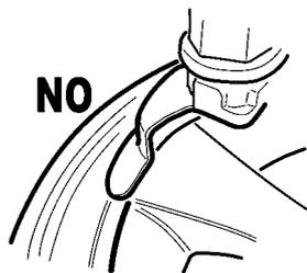
Bead incorrectly positioned causing bead damages between the head lip and the rim edge
