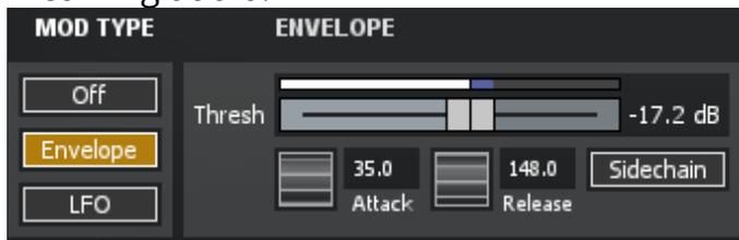
To setup an envelope sweep on a filter, select a filter and click the Envelope button under the Modulation tab.
