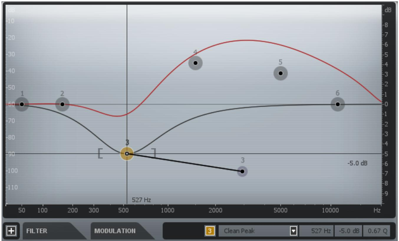
The Filter module provides six bands or filters as indicated by the six circle nodes on the spectrum. You can independently select and set each of these six filters, apply LFO or envelope effects, or change the type of each filter.
