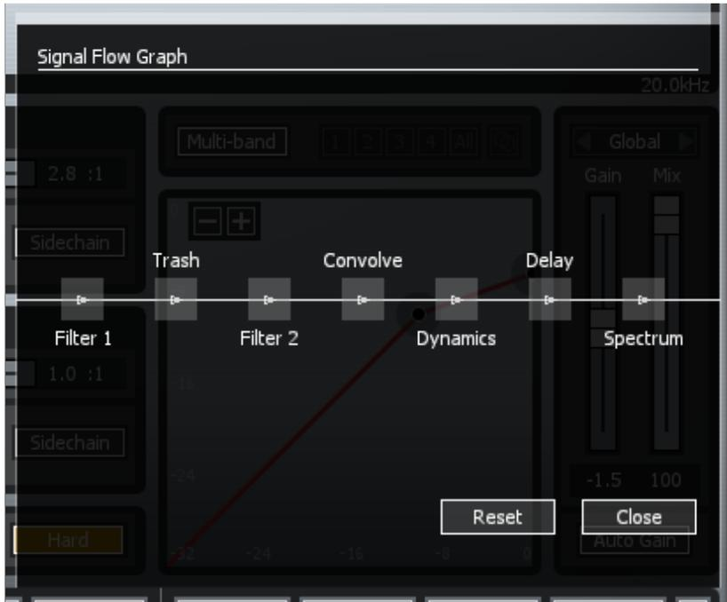
You can also place the spectrum anywhere within the processing, if for example you'd prefer to see a spectrum of the audio going into the Filter as opposed to seeing the spectrum after filtering.
