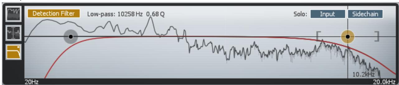
To enable the Detection Filter, select the third mini-spectrum view button in the top left of the window. Then, click the Detection Filter button that appears in the top left.
