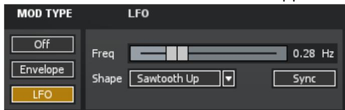
You can set the frequency of the sweep with the Freq control. Clicking on the waveform drop-down and selecting the desired waveform sets the shape.
