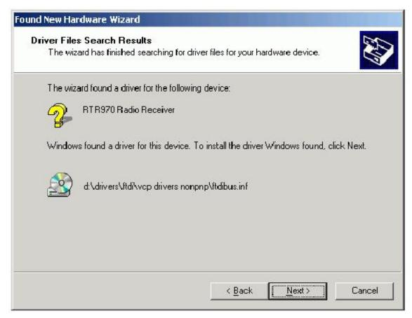
When USB bus driver ftdibus.inf is installed, Windows wants to install the virtual serial port driver, which makes the device look like an ordinary COM port.
