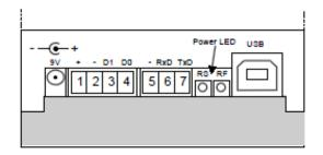
USB-, RS-485-, or RS-232-bus can be used to connect the device via serial communications. Each of these connections will be covered in their own chapter below. By default, the device is jumpered to use the USB-bus. If RS-485 or RS-232 -bus is to be used, the serial bus needs to be jumpered differently. Open the case by pressing in the fasteners on both sides of the RTR970 case. The case of FTR970 is opened by removing the screws
