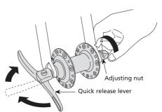
3. Grip the fork with your fingers and use the palm of your hand to close the quick release lever with as much strength as possible. When closed, the quick release lever must be in the "CLOSE" position shown below in the diagram on the right. The side of the lever with the inscription "CLOSE" must be facing away from the bicycle, and the lever should be parallel to the fork as shown below in the diagram on the left.
