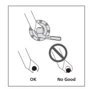
2. Open and close the quick release lever with your right hand while gradually tightening the adjusting nut with your left hand in the clockwise direction. Continue tightening the nut until you feel resistance with your hand at the point when the lever is parallel to the hub (as indicated by the dotted position in the diagram on the right)
