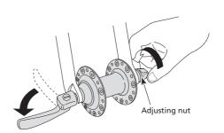
If the clamping strength is adjusted too strong and the quick release lever cannot be pushed to the CLOSE position, turn the adjusting nut in a counter-clockwise direction to reduce the clamping strength. When doing this, do not fully release the adjuster nut. Turn it 1/8 of a revolution, and then try to push the lever to CLOSE,
