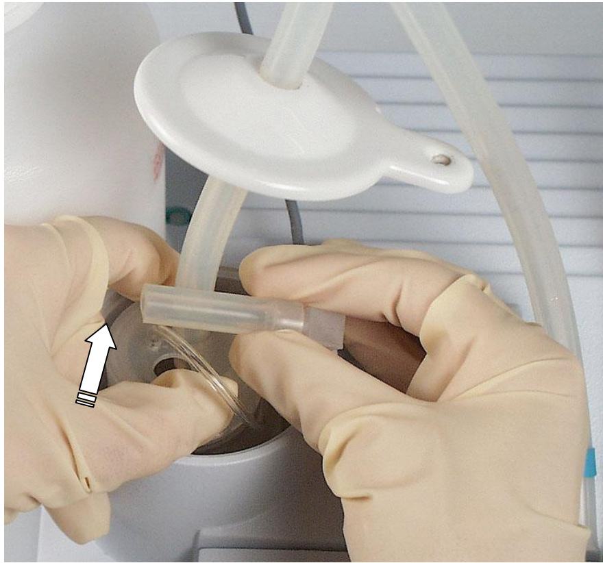
Fig. 7.3 Pulling the thick tube out of the liquid trap bottle
