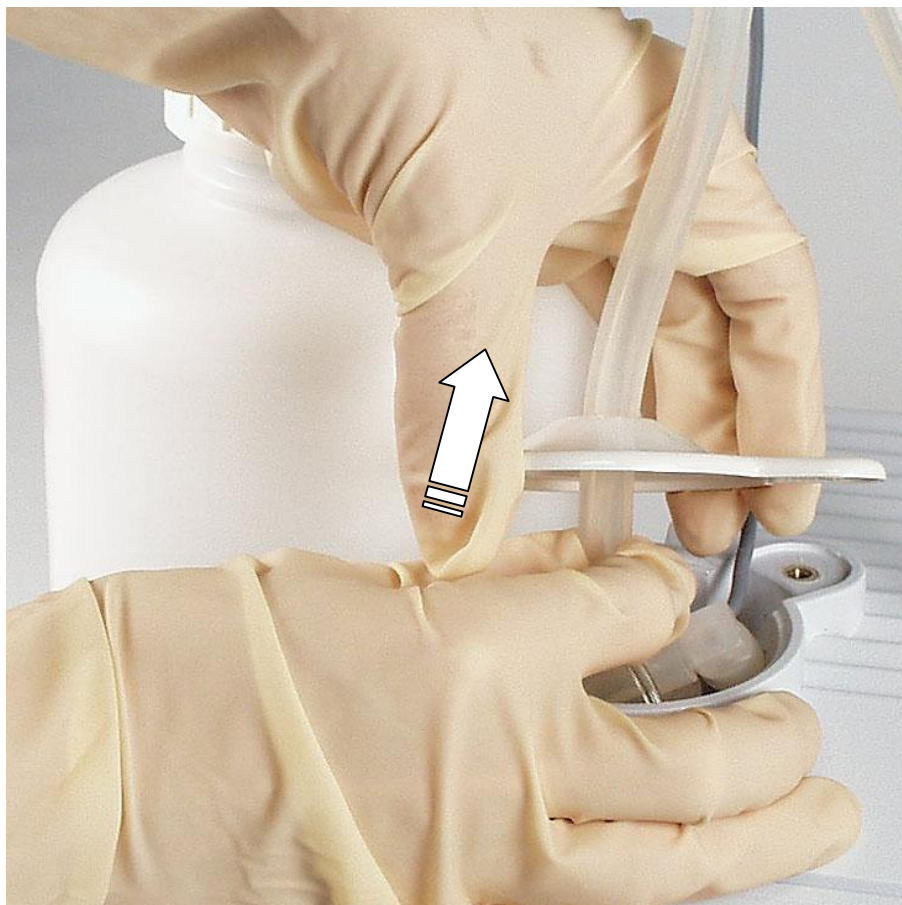
Fig. 7.2 Opening the liquid trap bottle cover
