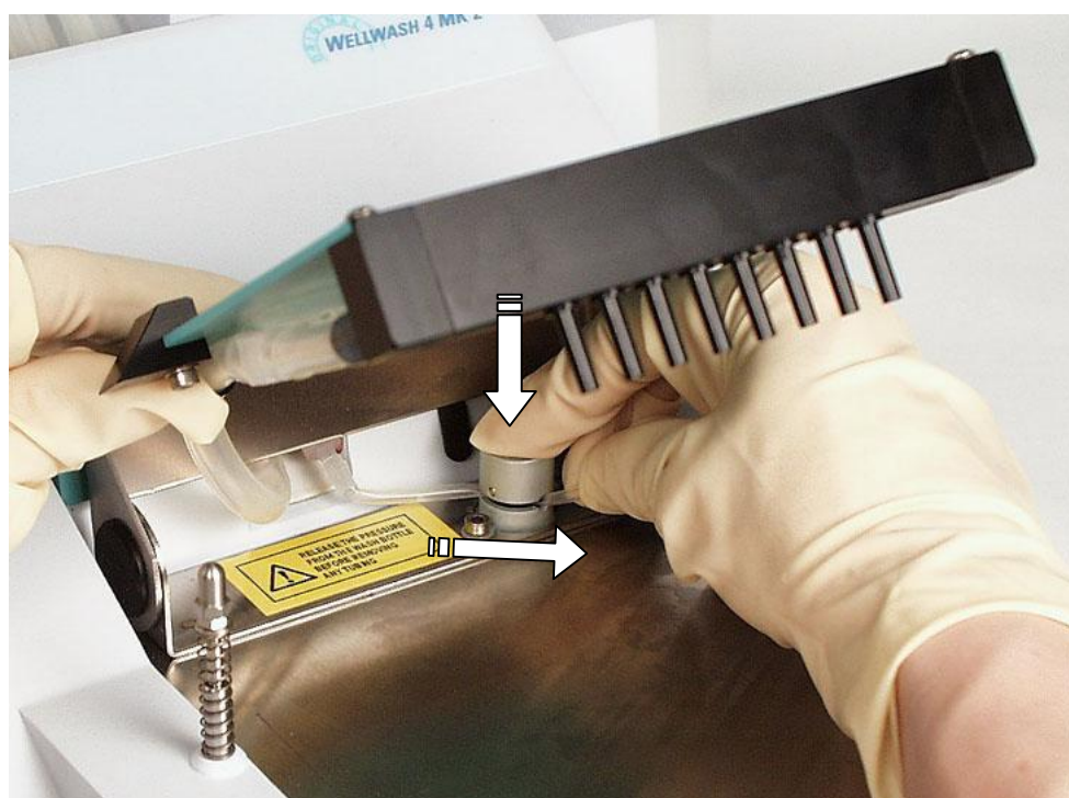
Fig. 7.6 Unpinching the tube
