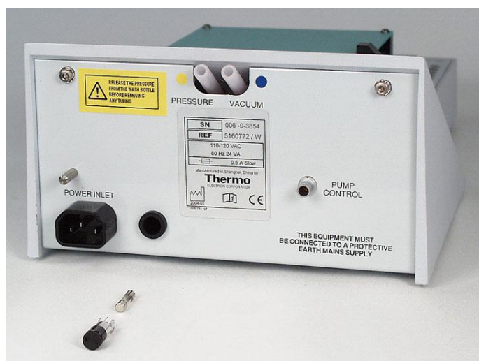
Fig. 7.9 Washer unit fuse and fuse holder
