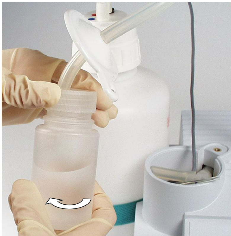
Fig. 7.5 Opening the liquid trap bottle
