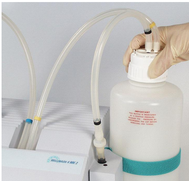
Fig. 6.1 Releasing the pressure from the wash bottle
