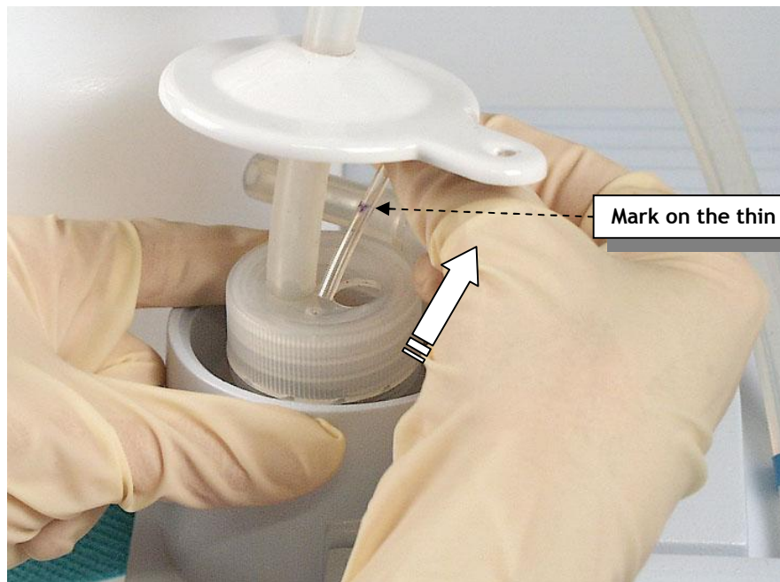
Fig. 7.4 Pulling the thin tube out of the liquid trap bottle
