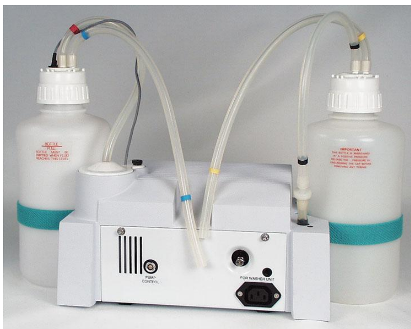
Fig. 5.8 Pump unit with tubes installed
