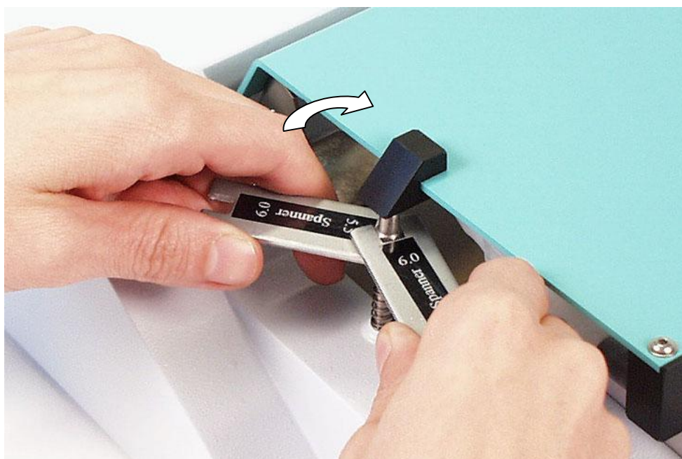
Fig. 5.14 Loosening the locknut with spanners
