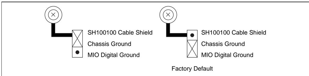
Figure 10-6. Ground Settings for SC-2056 Jumper W1
