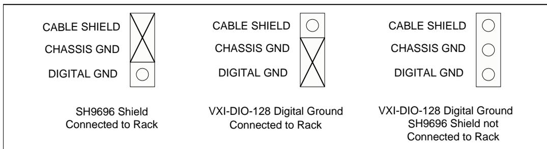
**Figure 10-8.** Ground Settings for SC-2057 Jumper W1
