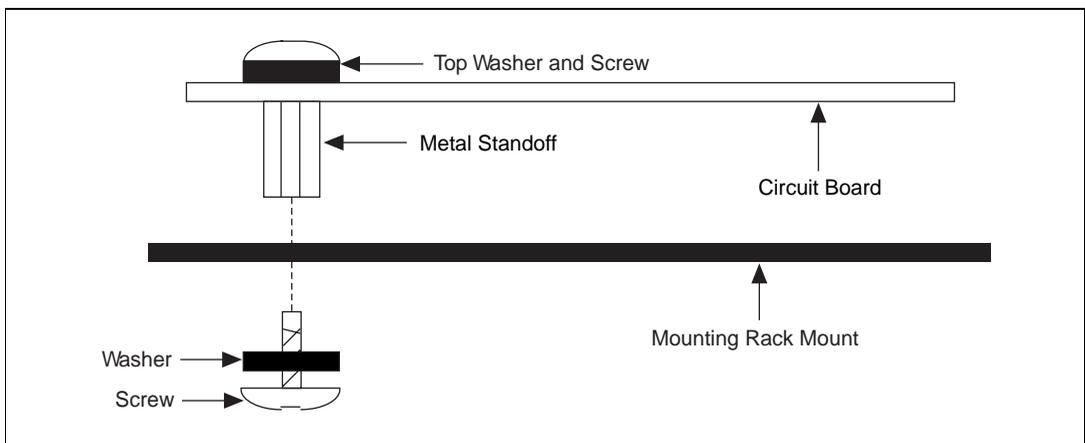
**Figure 10-2.** Attaching a Mountable Board to a Chassis
