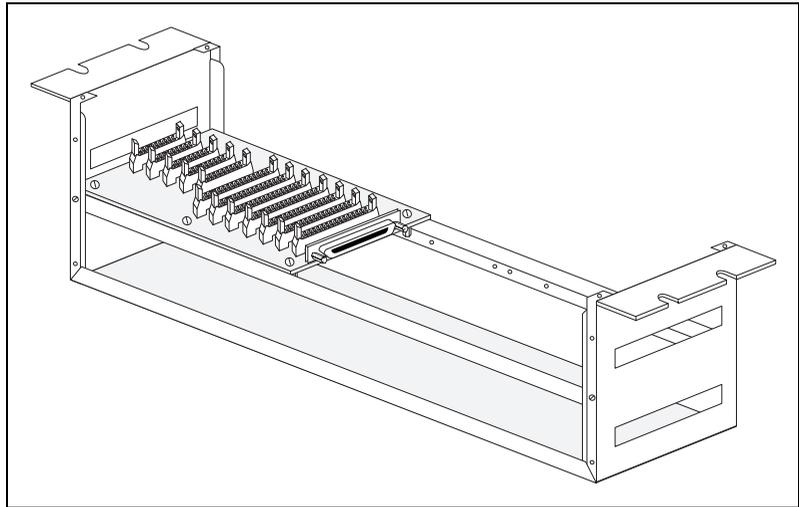
**Figure 10-1.** SC-2056 Adapter Mounted in a 19-in. Rack
