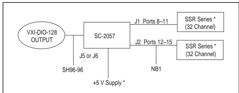
**Figure 9-4.** Output Connections with the 32 Channel SSR Backplane
