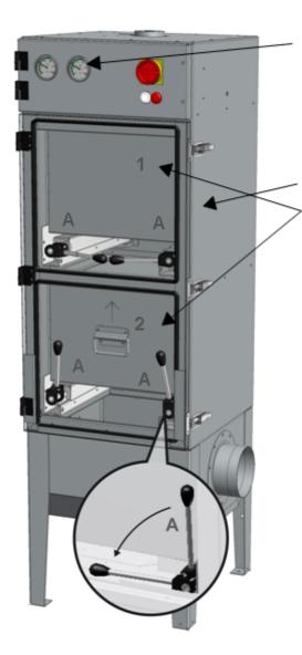
The pressure gauge will indicate the initial (clean) pressure of the system.
