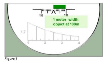
The windage scale engraved on the reticule is given in Mils (Figure 7). It can be used to make horizontal adjustments or as a rangefinder as well. The distance to the target can be determined by assuming that a 1m / 3'4" wide/long object fits between the small divisions at 100 m / 333 ft.
