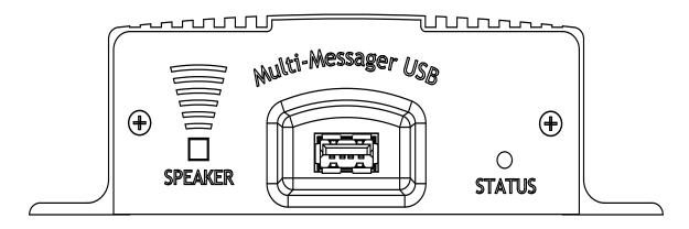
SPEAKER - The SPEAKER switch can be turned ON and OFF to monitor audio. The switch has no effect on the audio output connections on the rear of the unit. Switch should normally be kept OFF.
