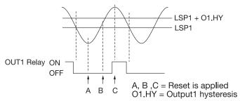
Figure 1.5 Low Limit Operation
