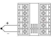
Figure 2.5 Thermocouple Input Wiring
