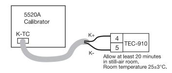
Figure 5.2 Cold Junction Calibration Setup
