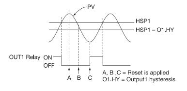
Figure 1.4 High Limit Operation
