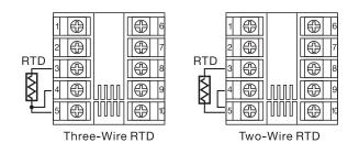
Figure 2.6 RTD Input Wiring
