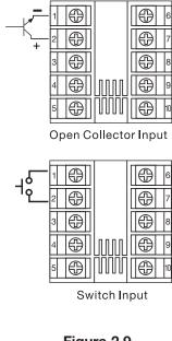
Figure 2.9 Event Input Wiring
