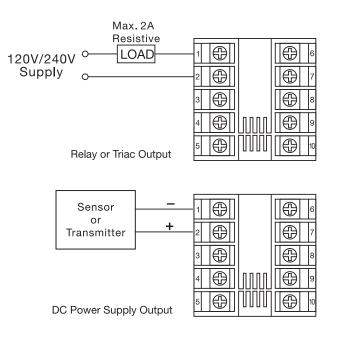
Figure 2.11 Output 2 Wiring
