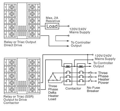
Figure 2.10 Output 1 Wiring
