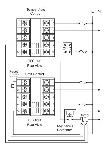
Figure 4.1 Over-Temperature Protection with Remote Reset
