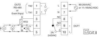
Notes: 50°C max. air ambient Use copper conductors (except on T/C input) ASTM thermocouples (USA), the red colored lead is always negative.
