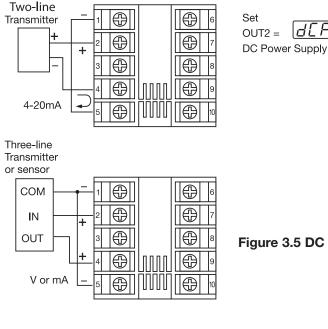
Figure 3.5 DC Power Supply Application
