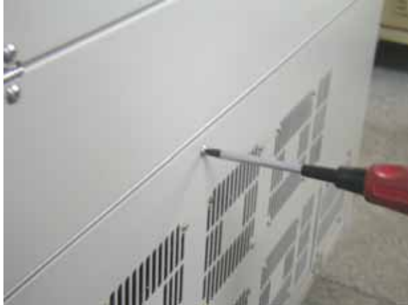
Fig. 4-2 Unscrew the Laser Cabinet
