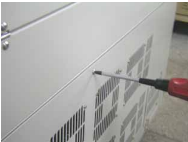
Fig. 4- 8 Screw the Laser Cabinet Panel to Finish the Power Cord Installation
