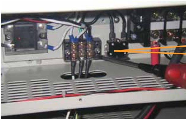
Fig. 4-7 Install the O shaped Cord to Terminal Connector
