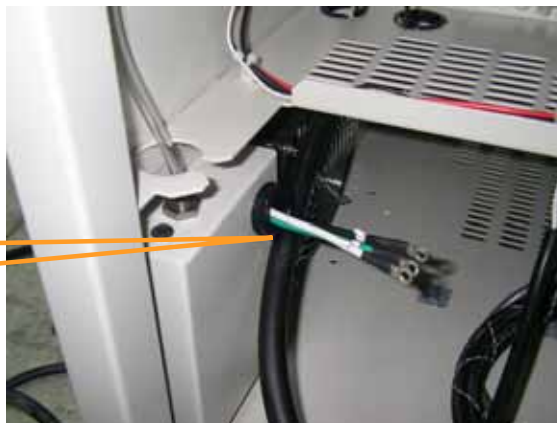
Fig. 4- 6 Install the Assembly and O ring to Spirit GE
