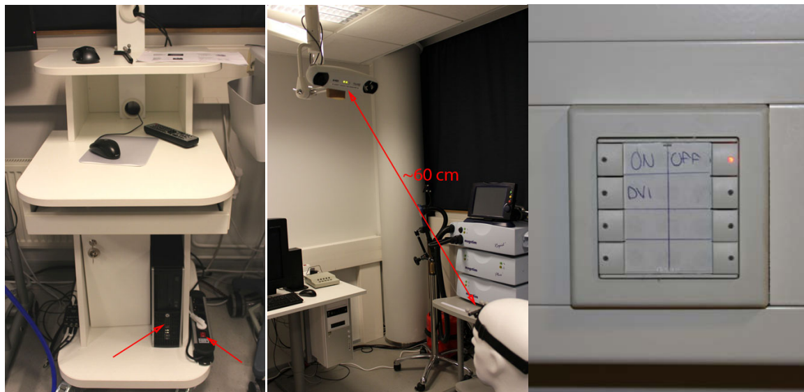
Figure 1. Visor2 neuronavigation computer,Polaris Vicra optical tracking system and power switch to the monitors. Extension cord power switch, computer power and optimal camera to reference tool distance illustrated.
