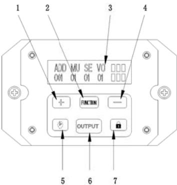
Plug the remote control into the rear of the smoke machine. Once the smoke machine is connected to the mains and switched on, the main switch will light indicating the unit is receiving power. The bar beneath the HEAT indication on the remote control display will blink. After a warm-up time of ± 5 minutes, the blinking bar will switch to OK, indicating the unit is ready.
