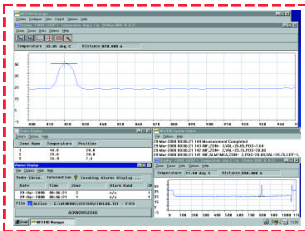
Figure 1 Illustrates the temperature profile display for the entire fibre length and also a numerical display for individual zonal temperatures.
