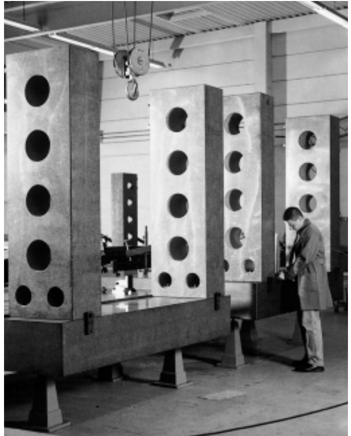
Assembly equipment for printing machines. Required evenness <math>< 0.008 \text{ mm}</math> over a surface area of 2700 mm x 2100 mm
