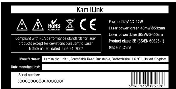
This sticker is placed on the bottom of the unit and gives further technical information including the laser power.
