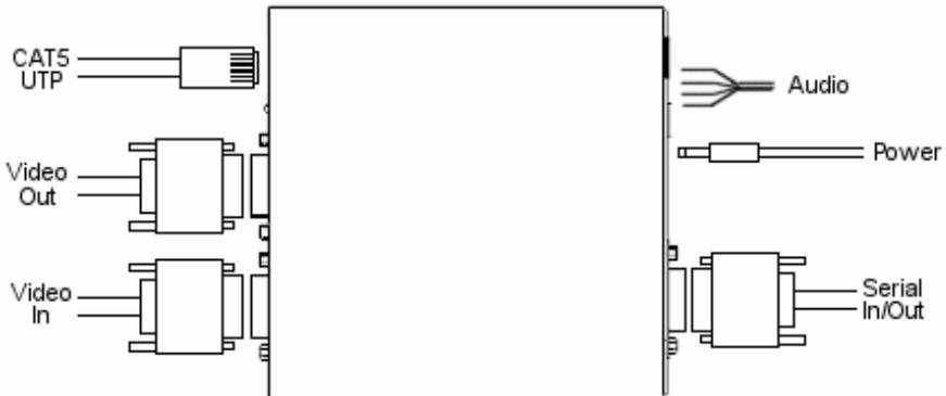
Figure 3: Transmitter Connections
