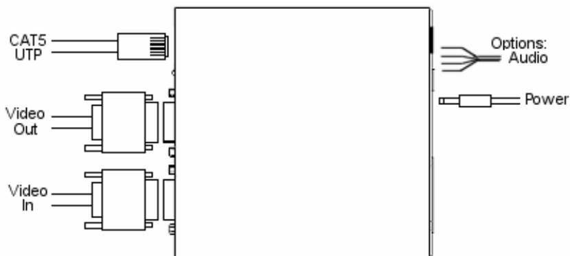
Figure 1: Transmitter Connections
