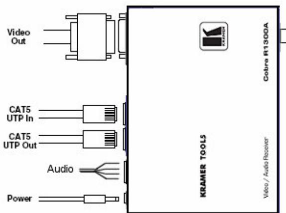
Figure 2: Cobra R1300A Video / Audio Receiver Connections
