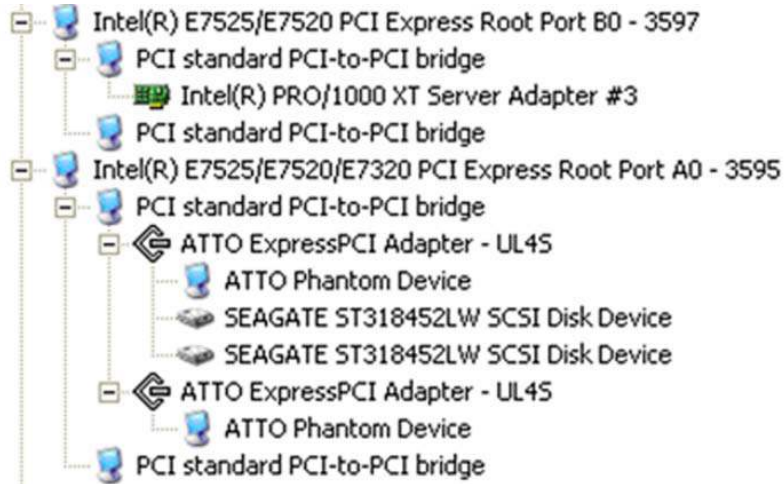
Windows Device Manager with 2 PCIe to PCI Expansion Systems Installed in a “Fan-Out Configuration.”
