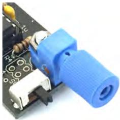
The interrupter set to live mode. Flip the switch to the left for fixed mode.
