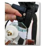
WARNING - AT EXTREME TILT ANGLES THE SHUTTER PLUG COULD HAVE INTERFERENCE WITH EMOTIMO PT. DURING PAN AND TILT MOVES ENSURE THERE IS NO INTERFERENCE BETWEEN THE PLUG AND EMOTIMO PT. THIS COULD DAMAGE THE EMOTIMO PT AND YOUR CAMERA!
