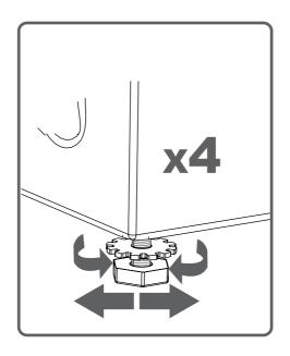
• Never put cardboard, wood or suchlike materials under your machine if you are intending to stabilize the distortions on the floor.
