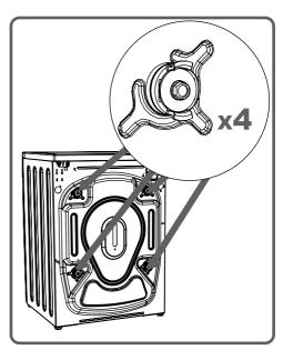
For this reason, transportation safety screws shall be loosened by being rotated in counter-clockwise using an appropriate spanner.
