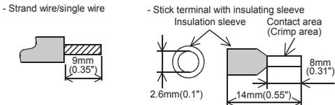
When using a stick terminal with insulating sleeve, choose a wire with proper cable sheath referring to the above outside dimensions, or otherwise, the wire cannot be inserted easily. The tightening torque must be 0.22 to 0.25 N·m. Do not tighten terminal screws exceeding the specified torque. Failure to do so may cause equipment failures or malfunctions.
