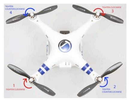
To attach the propellers, remove the warning discs from the motors and spin the propeller blades onto the corresponding motor in the direction indicated by the warning discs. Correct propeller installation is necessary for proper flight. Additional information can be found in the DJI User Manual.
