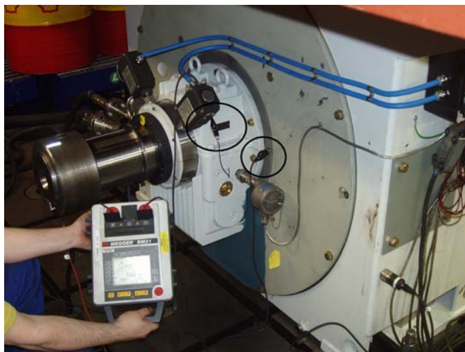
Figure 7-3 Measuring the insulation resistance of a sleeve bearing
