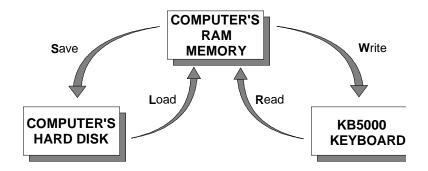
Dos shell File list (\*.tpl) Load file from disk Read from keybaord Save file to disk Write to keyboard Press ESC to Quit
