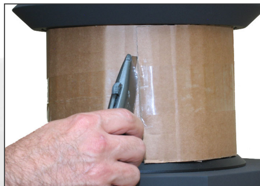
Figure 10. The Wrong Way to Remove a DDD Driver Cover
