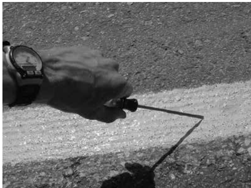
Figure 9—Check for Proper Cure
