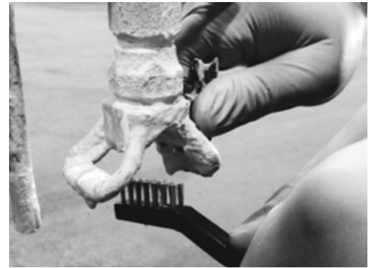
Figure 8—Clean the Spray Tip with a Brass Wire Brush
