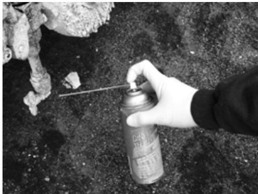
Figure 7—Clean the Spray Tip with Carburetor Cleaner
