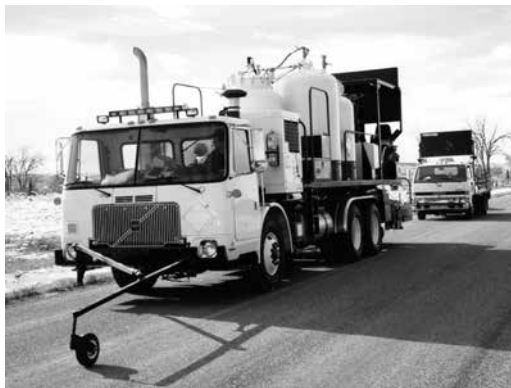
Figure 1 — LPM Application Truck
