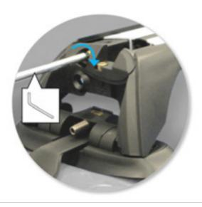
Tighten adjusting screw to 5 Nm.
