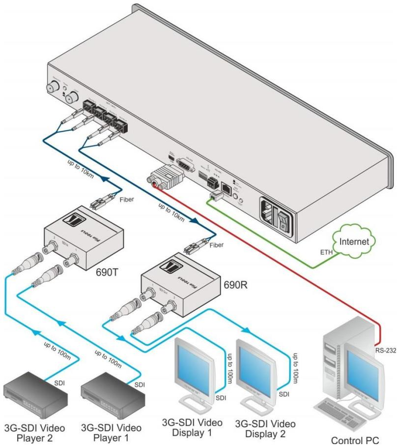
Figure 3: Connecting the VS-44FO
