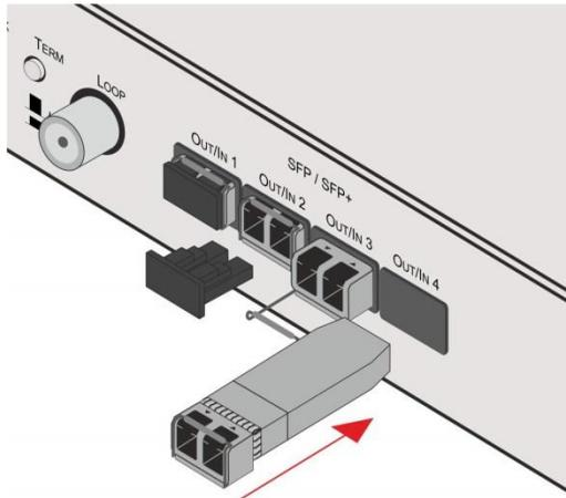
Figure 4: Installing the SFP Modules
