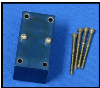
Figure 7.3-2: Four corner screws removed and scrubber removed from FROG
