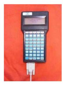
The unit used in this application is the QTERM-II <sup>™</sup> manufactured by QSI Corporation. The particular model chosen has a backlighted display, RS-232 9-pin "D" type connector, and the wide-temperature option. The alphanumeric display is four lines of twenty characters each. The unit has a forty (40) key tactile keypad; of which, five are user-definable. Five light-emitting-diode (LED) indicators are available for displaying status information in addition to the alphanumeric display.
