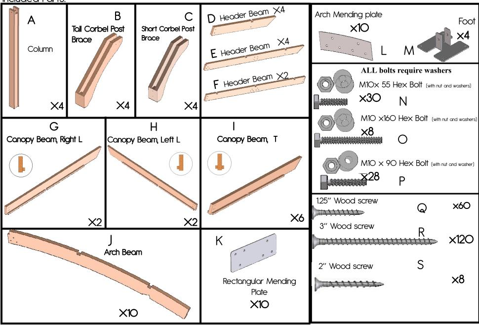
Step 1: Bolt steel footplate to each of four supplied posts "A" as shown. Use hardware "M", and "O".
