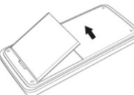
4. Hold your SIM card with the cut corner oriented as shown and then slide it into the card holder with the gold-coloured contacts facing downward.
