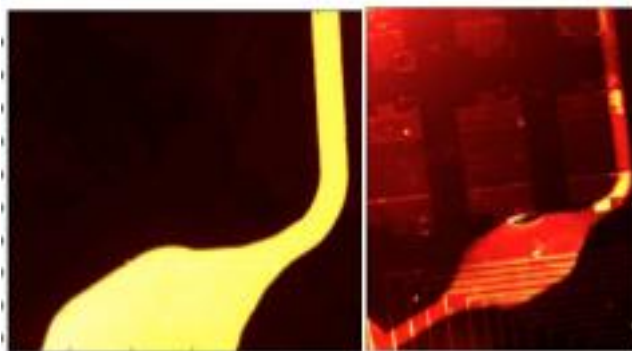
Figure IV-6; Fluorescing capillary fluid flow through permanently bound PDMS on glass slide (left) and fluorescing active fluid flow through permanently bound PDMS on LEAC chip (right)
