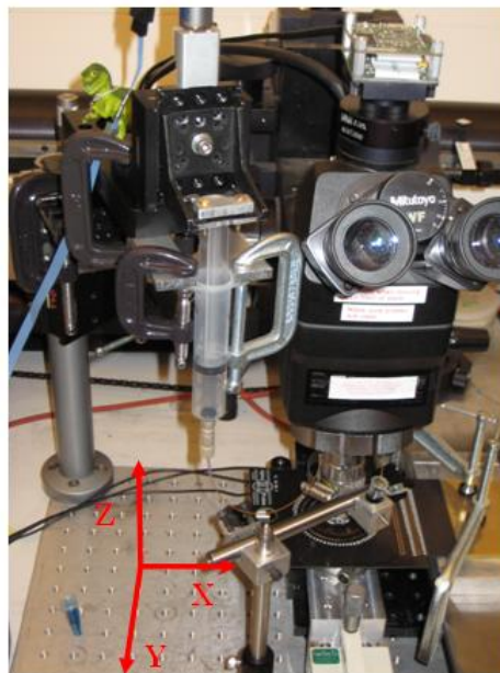
Figure A. 8: Coordinate definition for alignment instructions with the lucky testing dinosaur, Lenny
