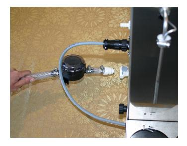
**NOTE:** To make sure there is no air in the flow path, turn the inline strainer upside down while the pump is running. This ensures that the air bubble in the strainer housing mostly dissolves, although a little air bubble in the strainer is normal.
