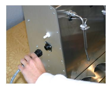
2.3 Plug the filler into a wall outlet. Turn on the Power Switch. **DO NOT** turn on the Pump Switch at this time.
