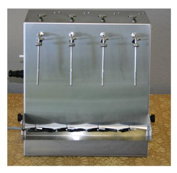
2.2 Unscrew the fixation screws holding the shelf to the machine body, and move the shelf to the bottom of the machine. Plug the electrical connector into the side of the filler (shown with optional gas sparge).
