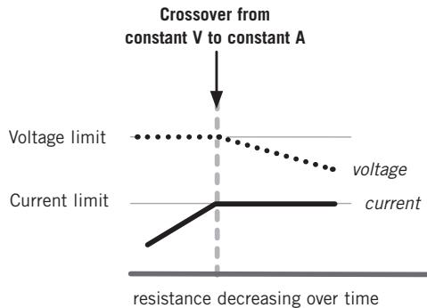
There are some conditions when the power supply will operate at the upper limit of 90 W of constant power. When this occurs, both the constant V and the constant mA lights will be lit at the same time.
