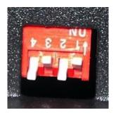
The factory settings correspond to 1 coin per credit. Switch 4 is not necessary.
