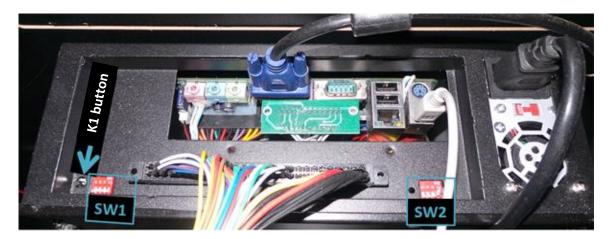
• A set of 4 switches on the left side called "SW1" to set up the coins needed to play, as explained below.
