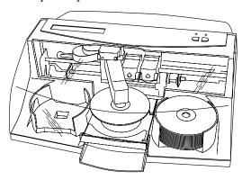
4. The Recorder Tray then automatically shuts. Robotic Disc Transporter will automatically check the Input Bin to make certain that only one disc was picked.
