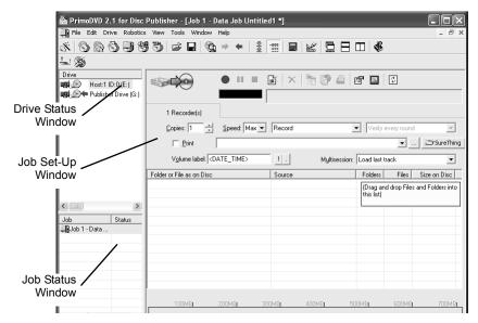
Under this window there are several adjustable-size windows that indicate what you've set-up and what's happening: the **Drive Status Window**, the **Job Status Window**, and the **Job Setup Window**. A sub-Window called the **Activity Log** is also available, but it is hidden upon initial boot-up of the software. Here's a short explanation of each Window:
