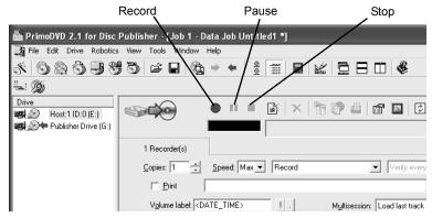
While jobs are running, they may be paused or stopped by clicking on the appropriate buttons on the Job Setup Panel. The Pause Button will allow the current recording to finish, then suspends operations on that job. Recording is resumed by clicking the Pause Button again.
