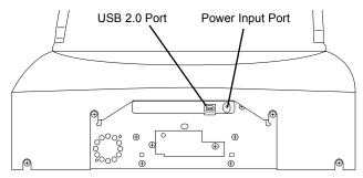
The USB 2.0 Interface is connected to an open USB 2.0 port on your PC with the USB 2.0 cable, included with your Publisher.
