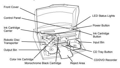
The **Robotic Disc Transporter** moves discs from the Input Bin, to a CD/DVD Recorder, to the printer, and finally to the Output Bin.
