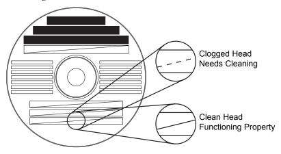
If the Yellow, Magenta, Cyan or Black diagonal lines printed on the disc show breaks, repeat the cleaning procedure. If nozzles still appear to be clogged, remove the cartridge and gently wipe the nozzle area sideways with a clean water-dampened cloth. If after several cleanings a color still does not appear on the test print, the cartridge may be damaged or empty and may need to be replaced.
