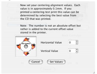
Look at the finished alignment disc and pick the numbers that come closest to lining up with one another. For instance, on the disc shown in this manual, the vertical alignment is 2 and the horizontal alignment is -3. Enter this in the alignment dialog box.
