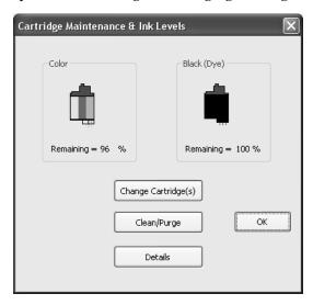
Select **Clean** button to send a simple test pattern to the printer. Be sure to have a disc in the Bravo's input bin and the front cover closed. The test pattern, shown below, purges ink through nozzles of your ink cartridge to clear any blockages. The test pattern will show if the nozzles require any further cleaning.
