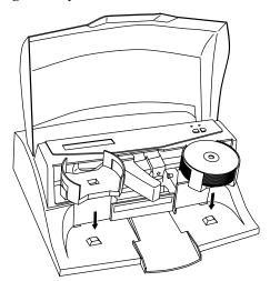
• Load the Input Bin (the bin located on the right-hand side of the Publisher) with 25 blank discs and place the bins on the mounting pegs.
