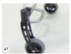
Provided that the seat height (front) should be retained, there must be a change of the angle by adjusting the position of the axle (vertical) and readjusting of the caster fork (right and left side) (49).
