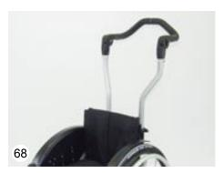
For transportation the push bar can be removed by loosening the cam lever or by pushing it inwards as far as it will go.
