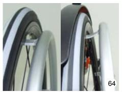
Hand rims can be supplied with a standard diameter (64, left) or with a larger diameter (64, right). These are called respectively hand rims "standard" or hand rims "high".
