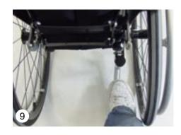
• Turn the anti-tip to the left as shown in illustration 10 (if the anti-tip is mounted on the left side turn it to the right side).
