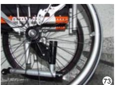
Adjust the anti-tipper so that it does not come in the way of the steps during transport. Afterwards, swing the antitipper back to its operational position.
