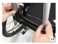
• Press in the spring button and slide the push bar (14) downwards fully into its bracket, until it clicks into position.
