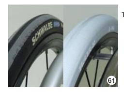
The drive wheels can also be supplied with solid PU-tyres (61, right).
