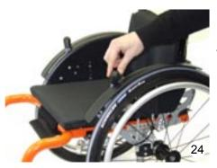
• To release the brake pull the brake lever upwards (24).
