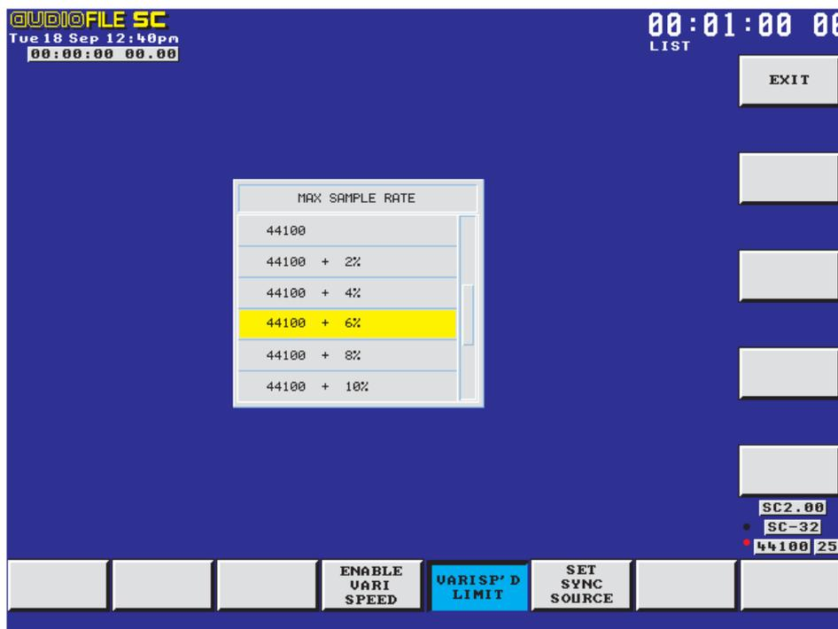
SET VARISPEED LIMIT allows the user to set the UPPER varispeed limit for the system sample rate and provides maximum processing resources. Use the left-hand softwheel to scroll through the options available. If varispeed is required it is advisable to set the maximum limit at the start of the session by pressing ENTER after selection - this will re-allocate the console.
