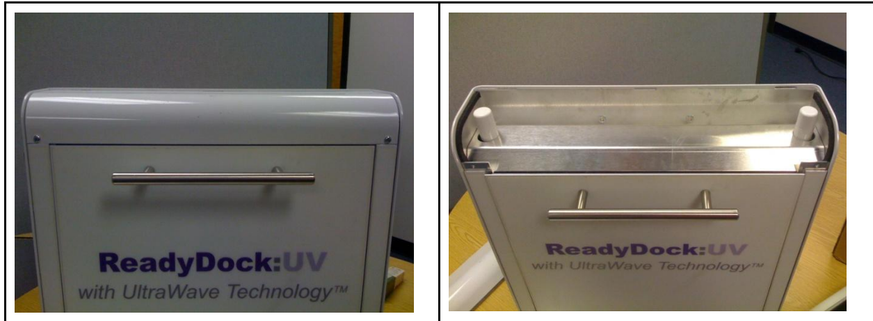
Figure 6 - Top Retaining Screw Location
