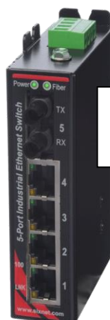
Typical ST style connector on a SL-5ES-2/3ST
