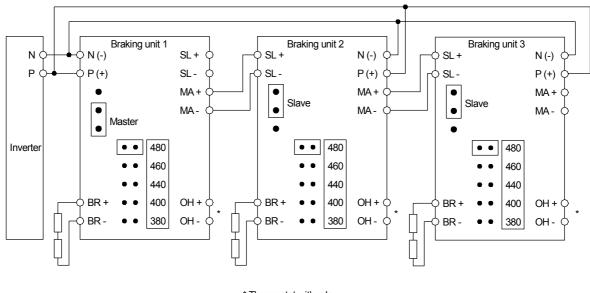
\* Thermostat with relay: 1A/125VAC 2A/30VDC For using multiple braking units need to parallel connected the barking units' main circuit terminal and selector the jumper 2(JP2) as follows:
