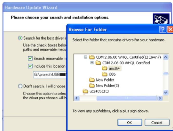
VII. Repeat 3 times install the driver for the port, It created 4 virtual serial port in the PC. The **Found New Hardware** balloon will reappear to inform you that the hardware was installed successfully. You can see them in Device Manager as follows(COM4~COM7):
