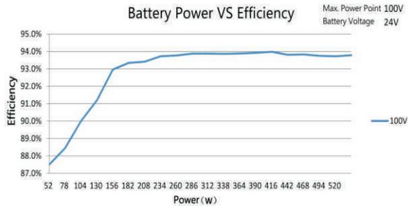
3. The MPPT tracing efficiency test (under the shaded condition).
