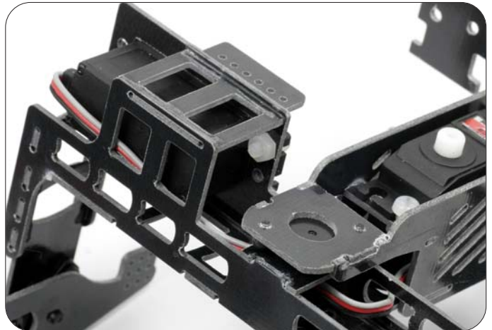
Pay attention to the trend of the servo wire (the trend of the servo wire in above picture is recommended)
