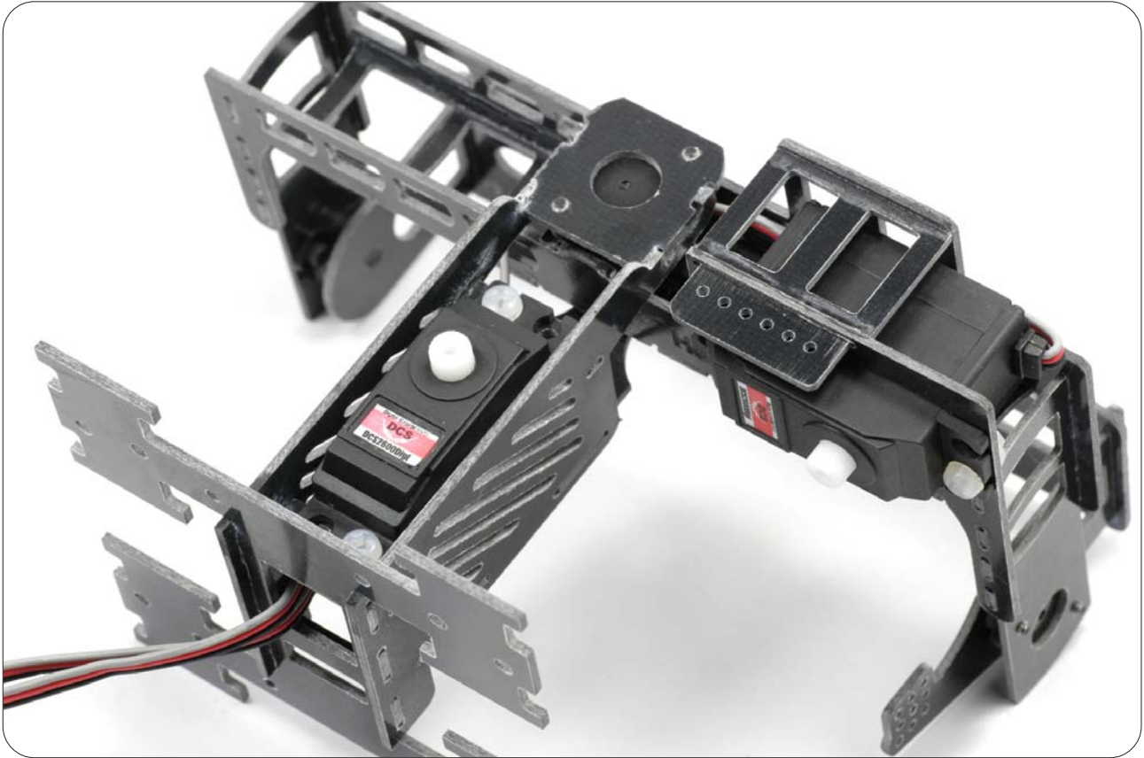
This is the installation of roll servo (Pay attention to the direction of the servo output shaft)
