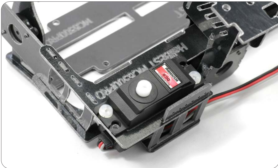
Using 2 nylon screws to fix the servo Install the servo as the picture above this is the installation method of pitch control servo
