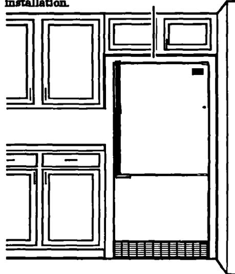
The refrigerator can be flush against the back wall.
